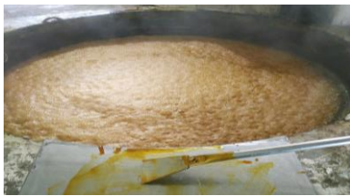
Concentration in open pan using vegetative clarificants
