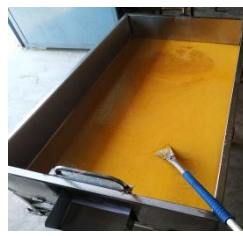
Concentration in open pan using vegetative clarificants
