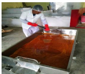
Concentration in open pan using vegetative clarificants
